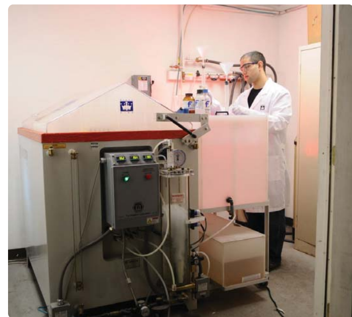
Industrial Rivet’s robust quality department includes in-house salt spray testing.
