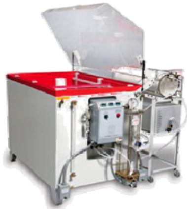
We employ Singleton® Salt Fog Chambers, Model SCCH-22
