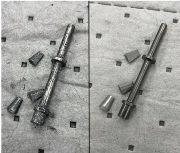
JAWS AND PUSHER SHOULD BE SHINING AND CLEAN WITH REGULAR SIMPLE MAINTENANCE. THE LEFT SET HAS NOT BEEN CLEANED, AND IS COVERED IN SMUT AND SWARF
