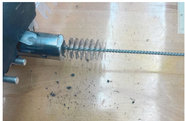
BLIND RIVET TOOLS USED AT HIGH PRODUCTION VOLUME REQUIRE REGULAR CLEANING TO REMOVE DEBRIS
