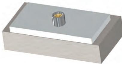
**Grooved Rivets:** When riveting inside a blind hole of plastic or wood material, the best solution is the grooved rivet. Annualar rings have been designed on the body so that the peak and valley of the groove embeds itself into the softer mating materials.
