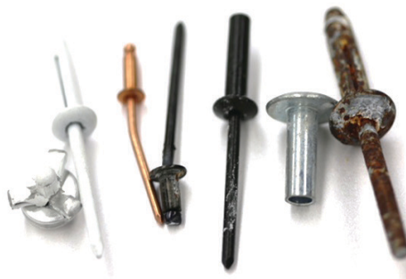
IMPROPER REPROCESSING CAN CAUSE RIVET FAILURE IN MANY WAYS INCLUDING CRACKING PAINT, BENT MANDRELS AND RUST.
